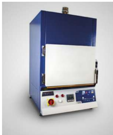
Bitumen content furnace by ignition method
