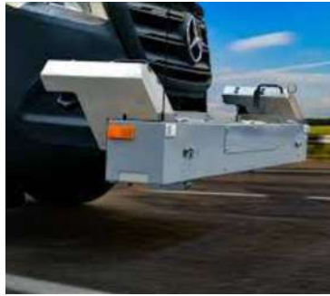
RSP III-Road Surface Profiler MK III
