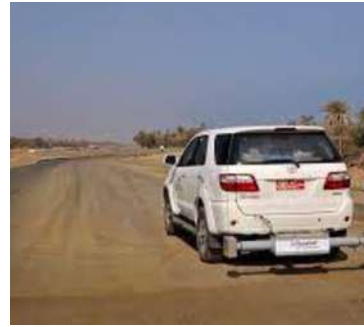
RSP IV - Road Surface Profiler MK IV
